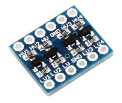
This bi-directional logic level converter is a small device that safely steps down 5V signals to 3.3V and steps up 3.3V to 5V at the same time. This level converter also works with 2.8V and 1.8V devices, with a total of four signals.
