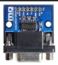
Using a MAX3232C transceiver, this serial adapter can operate with 3,3V and 5V digital signals (it also accepts 5V logic inputs with 3,3V supply). It meets the requirements of TIA/EIA-232-F and provides the electrical interface between an asynchronous communication controller and the serial port connector mounted on Pcs.
