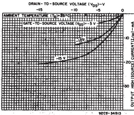
Fig. 2 - Typical output high (source) current characteristics.
