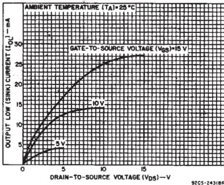
Fig. 5 - Typical output low (sink) current characteristics.
