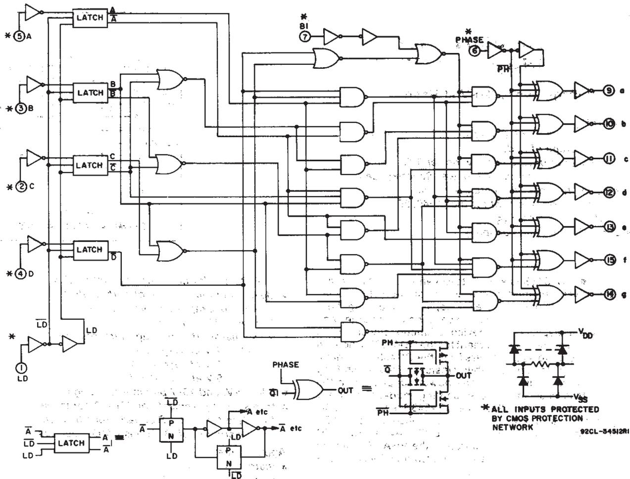
Fig. 1 - BCD-to-seven-segment latch/decoder/driver CD4543B logic circuit diagram.
