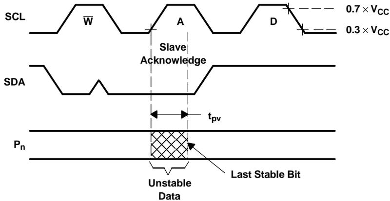
**Figure 3. Write-Mode Timing**
