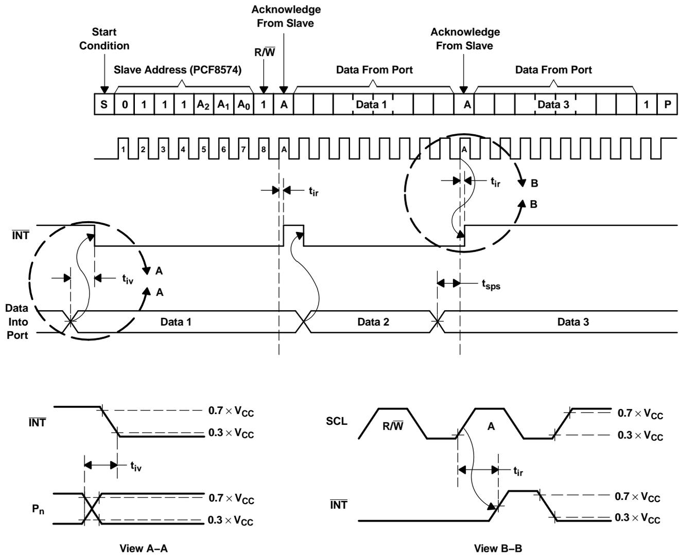
Figure 2. Interrupt-Timing Waveforms
