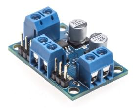
The *Dual DC Motor Driver 4A V3* allows to indipendently drive two DC motors, controlling both velocity and direction.
