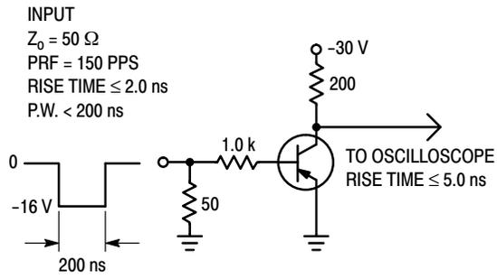
Figure 1. Delay and Rise Time Test Circuit
