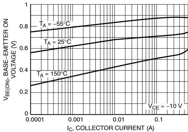
Figure 12. Base-Emitter Turn-ON Voltage vs. Collector Current
