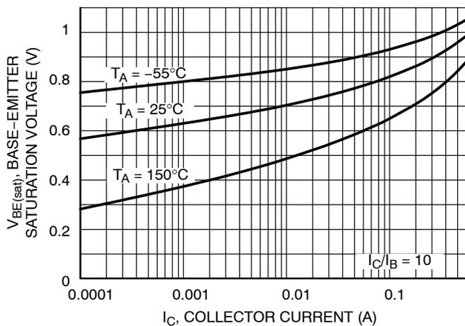
**Figure 13. Base Emitter Saturation Voltage vs. Collector Current**
