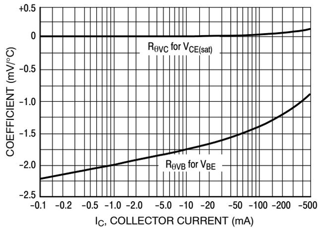
**Figure 14. Temperature Coefficients**
